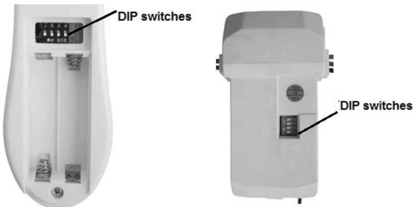
Fig. 11 Remote battery compartment
